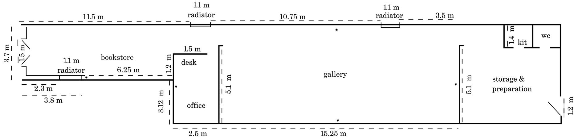
**Walls:** gyproc over 1.3 cm plywood continuous, not in contact with ceiling
